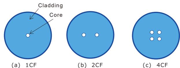
Fig. 4. Schematic cross section of a multi-core fiber
