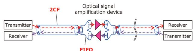
Fig. 5. Schematic diagram of a transmission system applying 2CF
