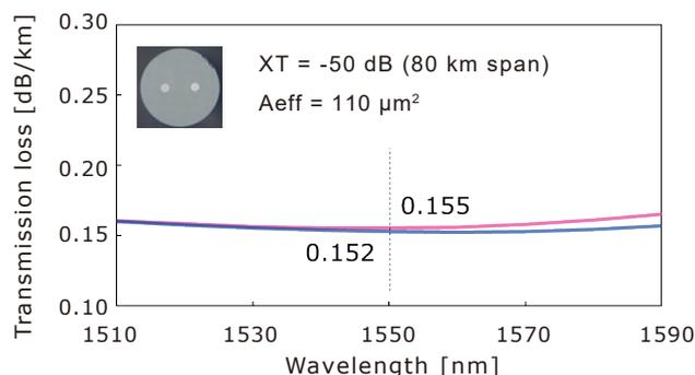
Fig. 7. Wavelength characteristics of 2CF transmission loss
